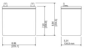
\*All dimensions in inches and (millimeters). All dimensions are for reference only. Contact a C&D Representative for complete dimensional information.
