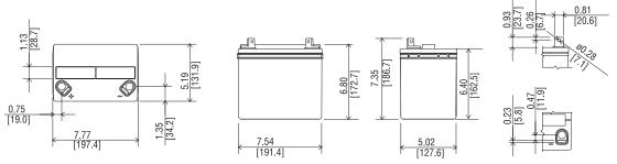
\*All dimensions in inches and (millimeters). All dimensions are for reference only. Contact a C&D Representative for complete dimensional information.
